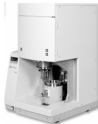
Figure 1. Diamond Dynamic mechanical analyzer (DMA)
