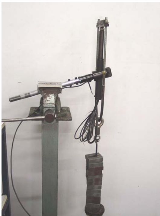
Figure 8. Calibration of the X force transducers
