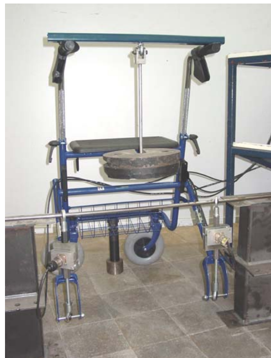
Figure 9. Calibration of the wheel transducers
