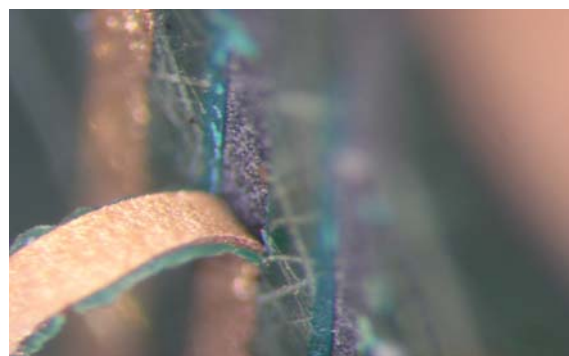
Figure 6. The laboratory separation of the conductive ways by temperature shock
