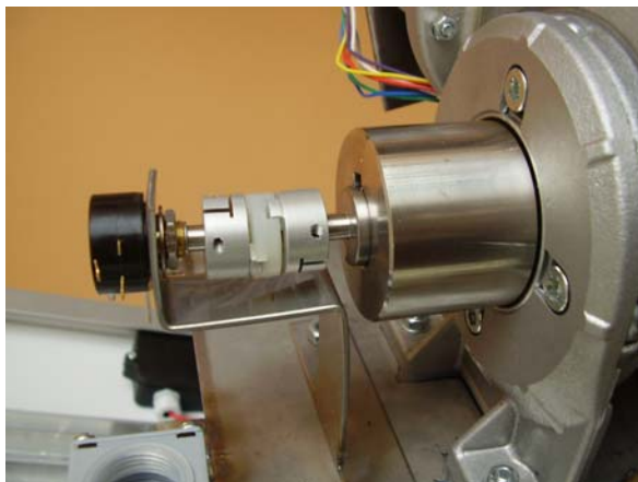
Figure 3: Measurement of position with potentiometer sensor
