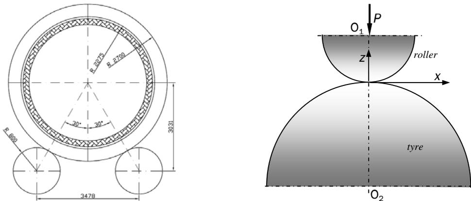
Figure 4. Tyre-roller contact: left – real geometry, right – simplified FE model
