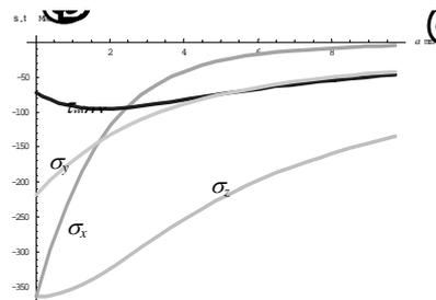
Figure 5. Stress distribution in the roller with corresponding expressions
