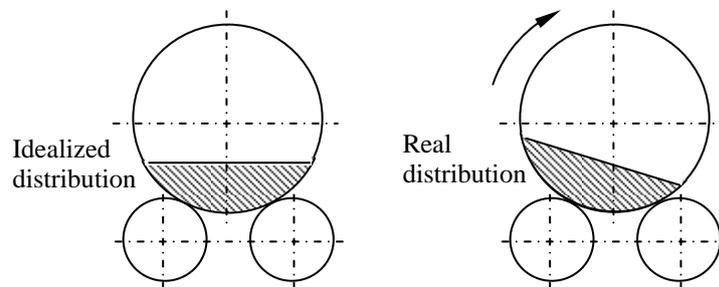
Figure 2. Distribution of raw-mix around vertical axis
