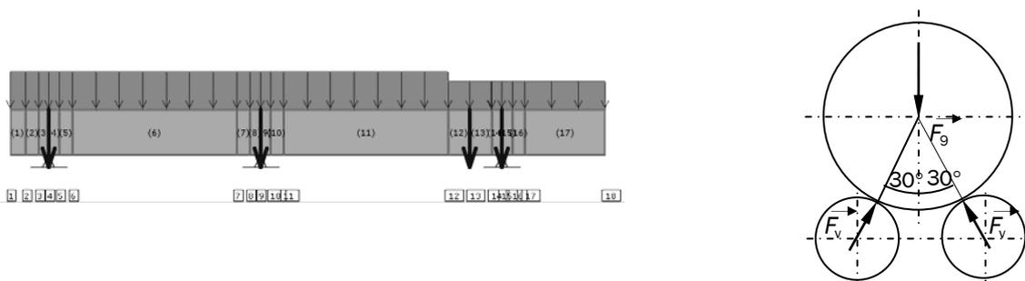
Figure 3. left - Kiln modeled as a cantilever beam, right - roller stations with reactions
