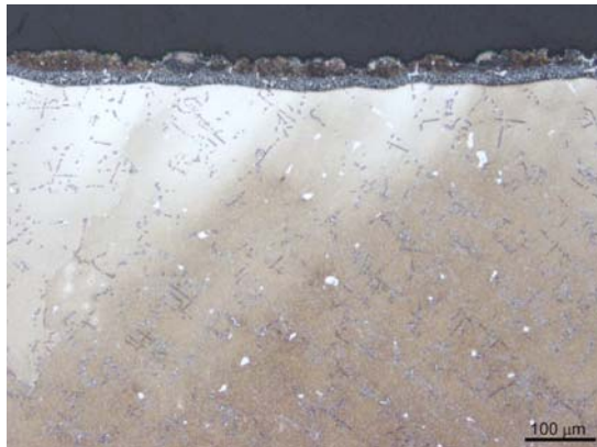
Figure 1a. Microstructure of Al-Si layer on ZHS6K (pressure spraying + diffusion annealing), LM
