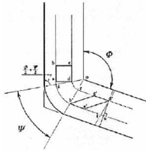
Figure 2. Dimensional parameters of the ECAP extruding channel
