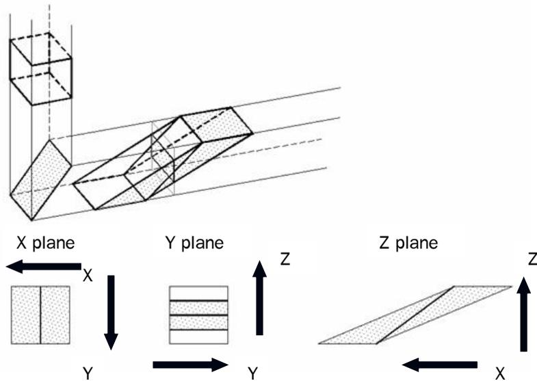
Figure 1. Principle of the ECAP technology
