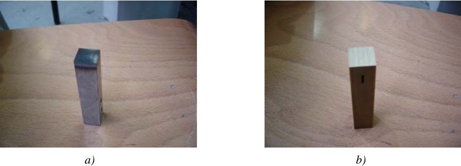
Figure 2. Surface of the work piece after grinding, a) construction steel, b) brass
