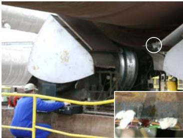
Figure 10. Strain gauge bonded on the ring
