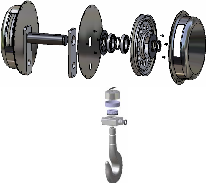
Figure 2. Formation of the lower sheave assembly
