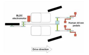
Figure 1. Principal construction of the HPV
