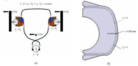
Figure 3. a) Steering by Bowden cables. b) The Adjusting rope-wheel.
