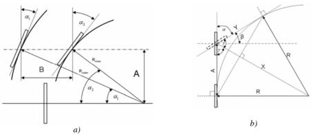
Figure 2. a) - 'Drive through a curve' conditions. b) - Geometry of turning.
