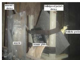
Figure 4. Impact between 14.5 x 114 mm calibre piercing incendiary bullets and configuration constituted by 6 mm thickness armour plate and bulletproof jacket
