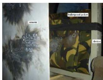
Figure 2. Impact between 7.62 x 54 mm calibre piercing incendiary bullets and configuration constituted by 6 mm thickness armour plate and bulletproof jacket
