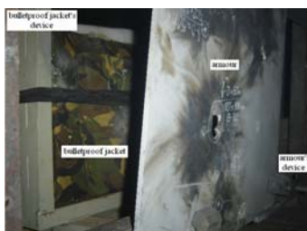
Figure 3. Impact between 12.7 x 108 mm calibre piercing incendiary bullets and configuration constituted by 6 mm thickness armour plate and bulletproof jacket
