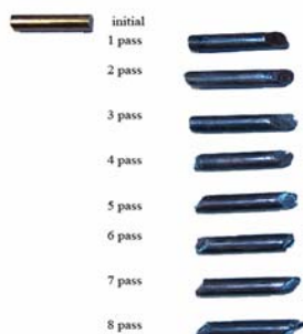
Figure 2. Copper samples after individual passes with use of the ECAP technology
