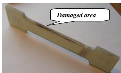
Figure 7. Degradation of the material during immersion in water
