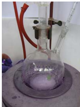
Figure 1. Heating balloon with column for rectification [3]
