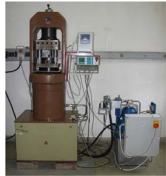
Figure 3. Working site for verification of new geometry of the ECAP tool
