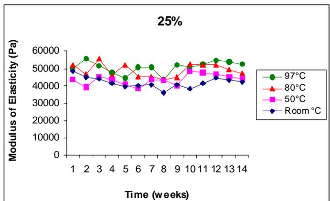
Figure 5. Variation of elastic modulus with swelling time in 25% solution
