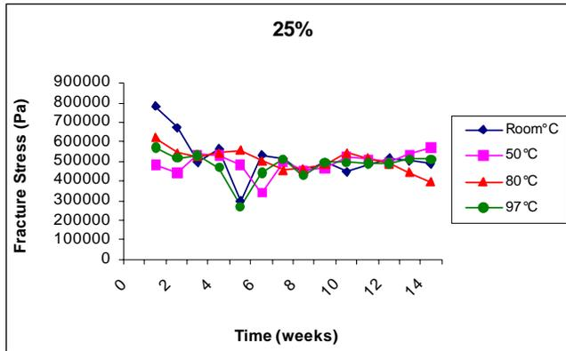
Figure 3. Variation of fracture stress with swelling time in 25% solution
