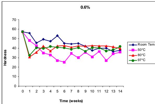
Figure 1. Variation of hardness with swelling time in 0.6% solution
