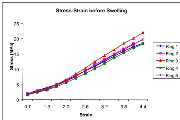
Figure 2. Stress-strain behavior of 5 ring samples before-swelling
