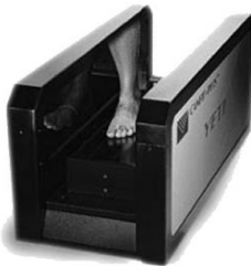
Photo 1: Alpina's first optical foot measuring instrument, called Yeti
