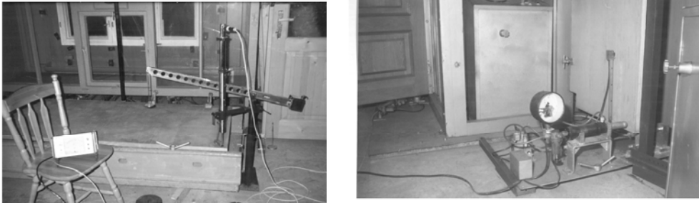
Figure 3 Installations for testing the sheet doors at bending on the horizontal plane (left) and on the vertical plane (right)
