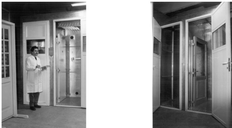
Figure 5 Automated climatic chamber for testing the doors and windows at temperature and humidity variations
