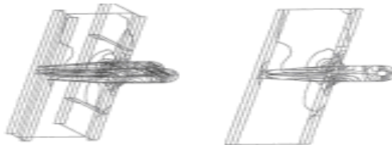
Figure 5. Stress distribution, 0-8.4 step 0.8 kN/cm 2
