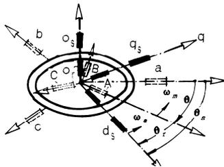
Figure 3. d-q frame in IM
