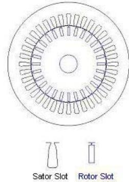
Figure 2. Cross section of IM, stator and rotor
