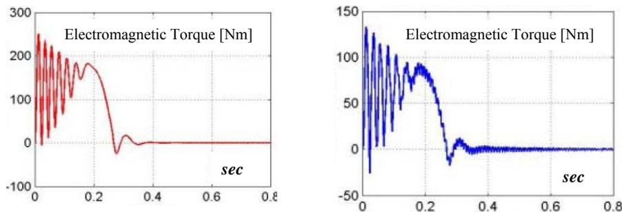
Figure 7. Squirrel-cage induction motor 7.5KW, 340V delta-connected, 50 Hz, 1400 rpm, 9.2 A, four-pole: electromagnetic torque [Nm], without skin effect (left) and with skin effect (right)
