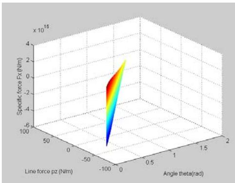
Figure 4. Line and specific x-axe force vs. dislocation angle
