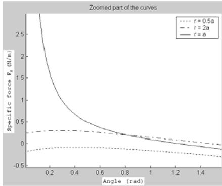
Figure 2. Specific force in x-direction vs. dislocation angle
