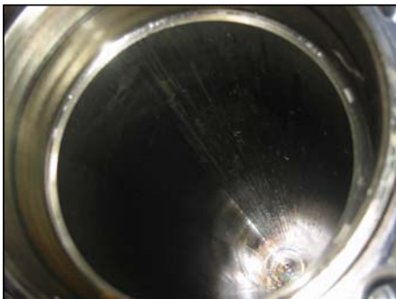
Picture 3. Damages of boom cylinders
