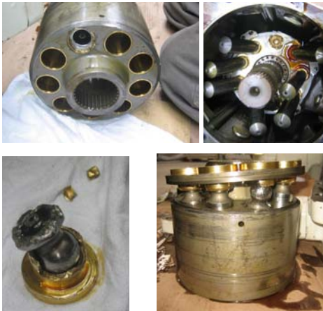
Picture 2. Damages of pump No. 2 elements
