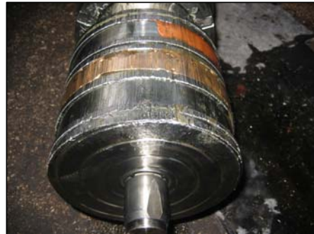
Picture 3. Damages of boom cylinders
