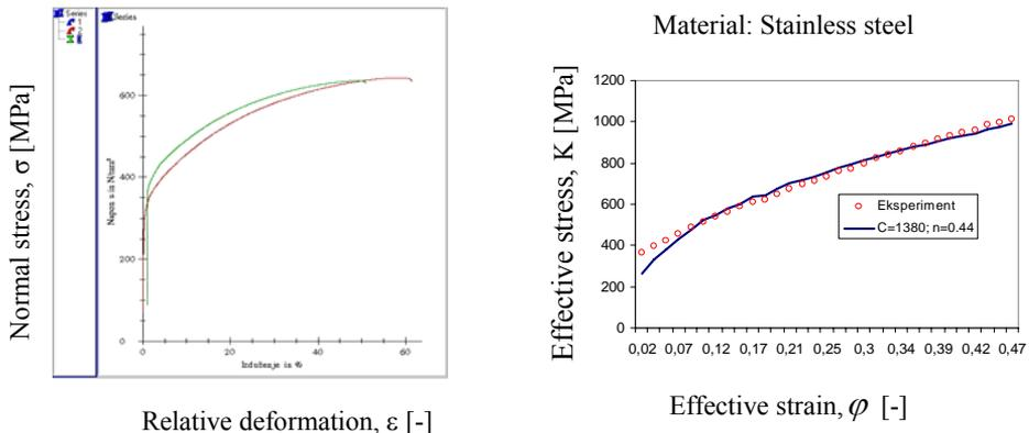
Figure 1 The results of uniaxial tensile test and yield stress for stainless steel INOX X5CrNi18-10
