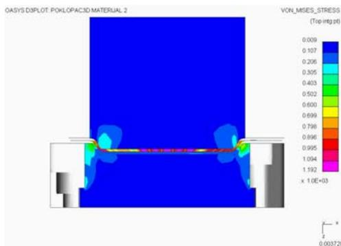
Figure 3. Von-Mises stresses and strains of punch, die and lid
