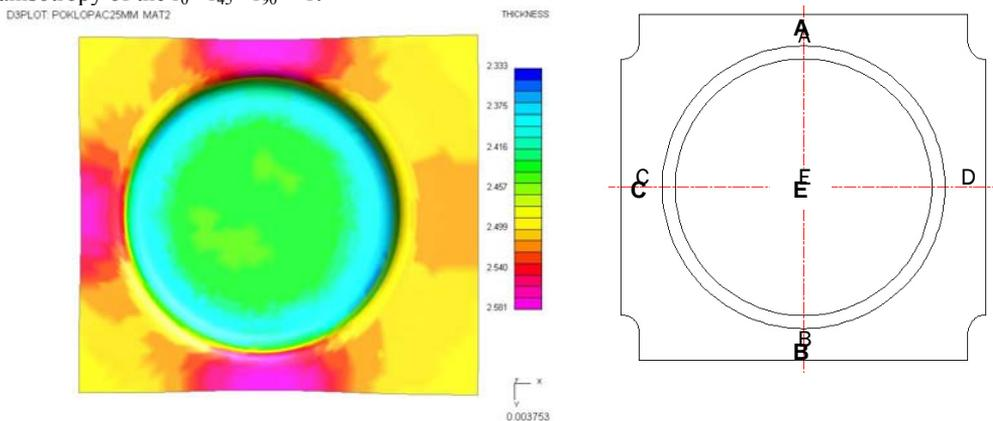
a) Changes in the thickness on the numerical model      b) Position of measuring points
