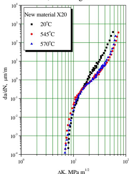
Fig. 1: Diagram of dependence  $da/dN$ - $\Delta K$  for the specimens taken from new pipes made of steel X20
