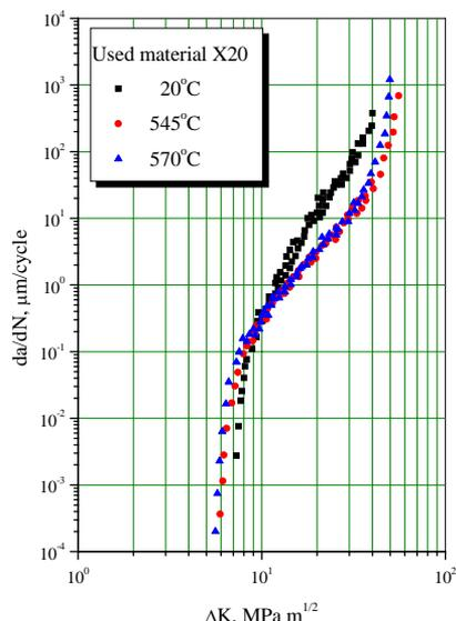
Fig. 2: Diagram of dependence  $da/dN$ - $\Delta K$  for the specimens taken from used pipe made of steel X20
