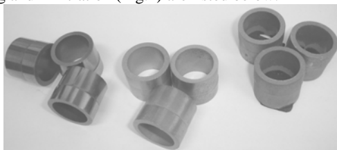
Figure 1. Iron-copper details after compacting, sintering and infiltration.
