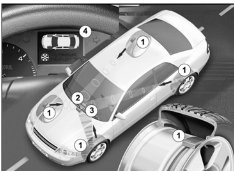
1-pressure sensor, 2-receiver, 3-electronic control unit, 4-display unit Picture 1. Tyre pressure monitoring system
