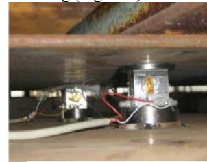
Figure 7. Dynamometers for measuring press force[5]
