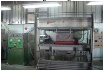
Figure 5. Hydraulic presse with generator of VF- electricity [5]
