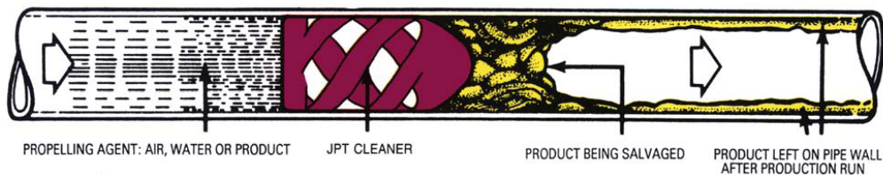
Figure 3. Method of pigging
