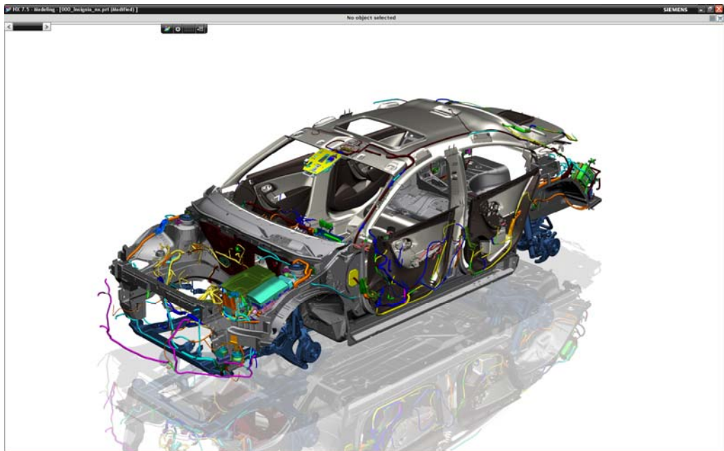
Figure 17. With the actual CAD systems the designers can create a single digital model with the possibility to design, visualize, and simulate their products.
