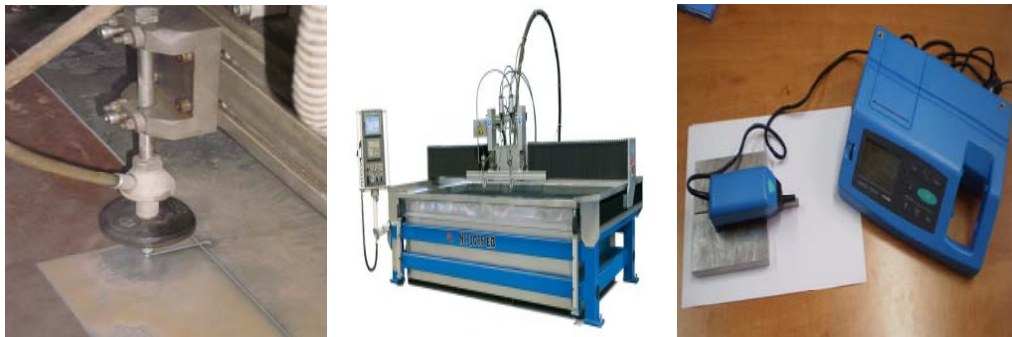
Figure 1. Cutting of the sample, machine NC3015 and measuring of surface roughness on the machine T1000 basic
