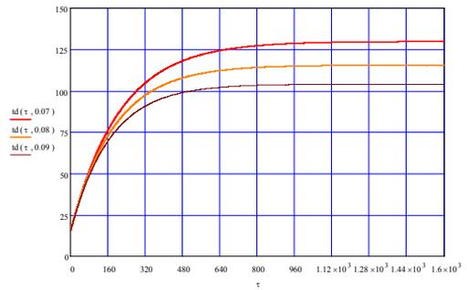
Figure 4. Temperature at the exit of fluid depending on the time and the mass inflow
