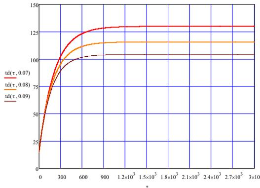
Figure 5. Temperature at the exit of fluid depending on the time and the mass inflow
