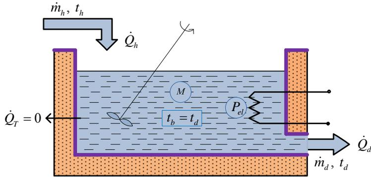
Figure 1. Isolated directly Heat exchangers
