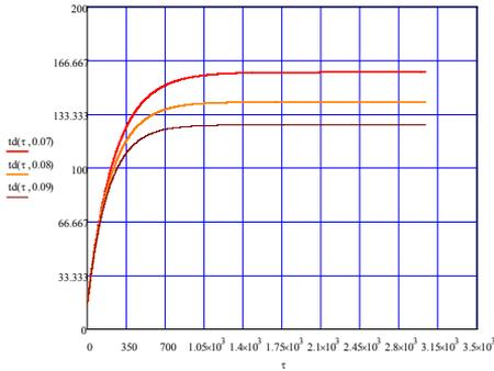
Figure 3. Temperature at the exit of fluid depending on the time and mass inflow
