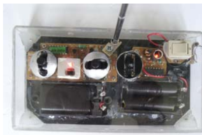
Figure 5. Control electronics (Receiver and Transmitter platest
