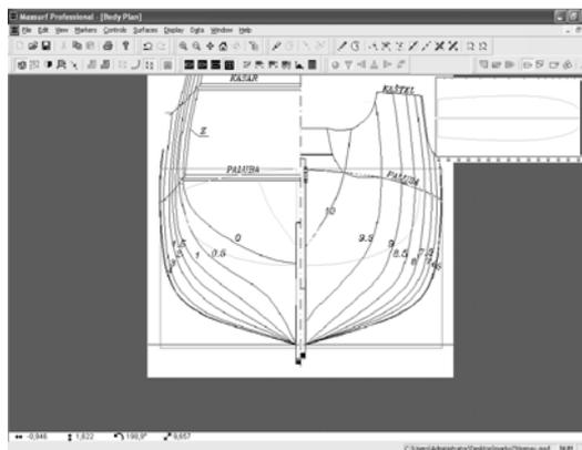
Figure 3. Body plan (hull lines) in Maxsurf
