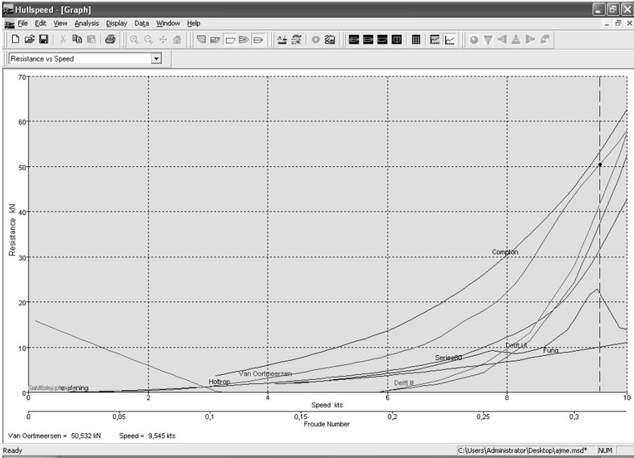
Figure 5. Results of the hull resistance calculation (Hullspeed)
