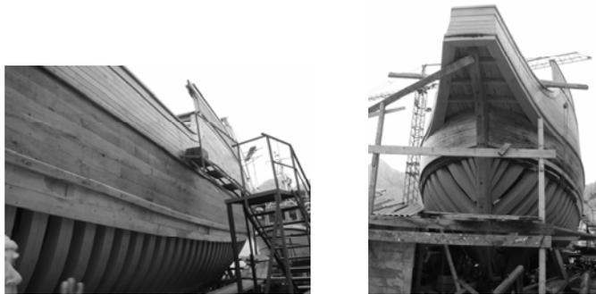
Figure 2. Building site and wooden structure of galleon 'Tirena'
