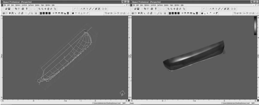
Figure 4. CAD model of galleon 'Tirena'. Left: wireframe model; Right: 3D model
