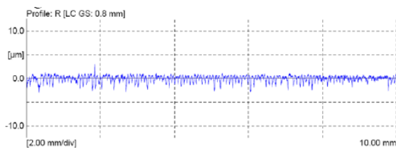
Figure 2 Surface characteristic of shaft
