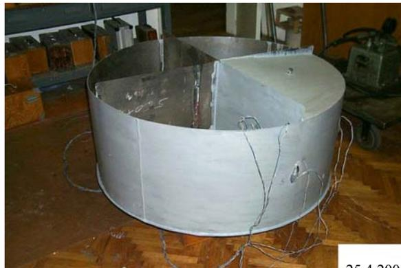
Picture 1. Model of the vertical cylindrical tank with partitions
