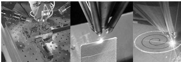
Figure 1. Directed Metal Deposition: a) RP workstation, b) i c) creating layers [2]
