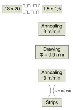
Figure 1. Schematic presentation of the experimental procedure
