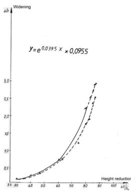
Figure 2. Dependence of widening on height reduction
