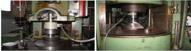
Figure 1. The experimental tool located in the eccentric and hydraulic presses with the equipments for the presentation of the force and the working foot.
