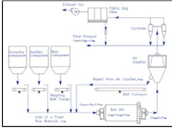
Figure 1. Flow sheet of a grinding plant
