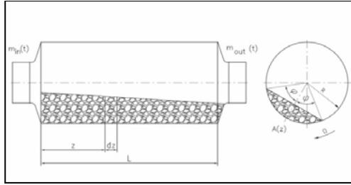
Figure 2. Distribution of the mass inside the ball mill
