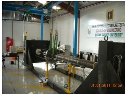
Figure 2. Solid expandable tubular test rig at Sultan Qaboos University, Muscat
