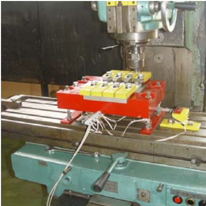
Figure 4. Machine performing FSW.
