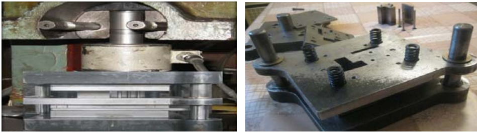
Figure 3. The experimental tool located in the eccentric presses with the equipments for the presentation of the force and the working foot.
