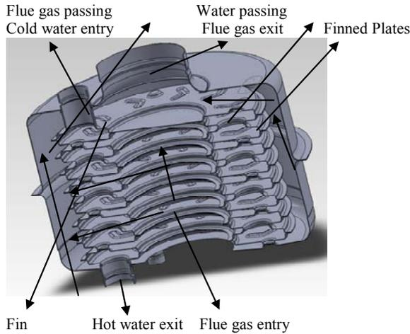
Figure 1. The cross-section of the multi passage compact heat exchanger
