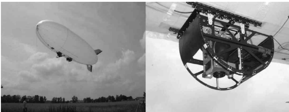
Figure 3. The airship with the thermographic camera
