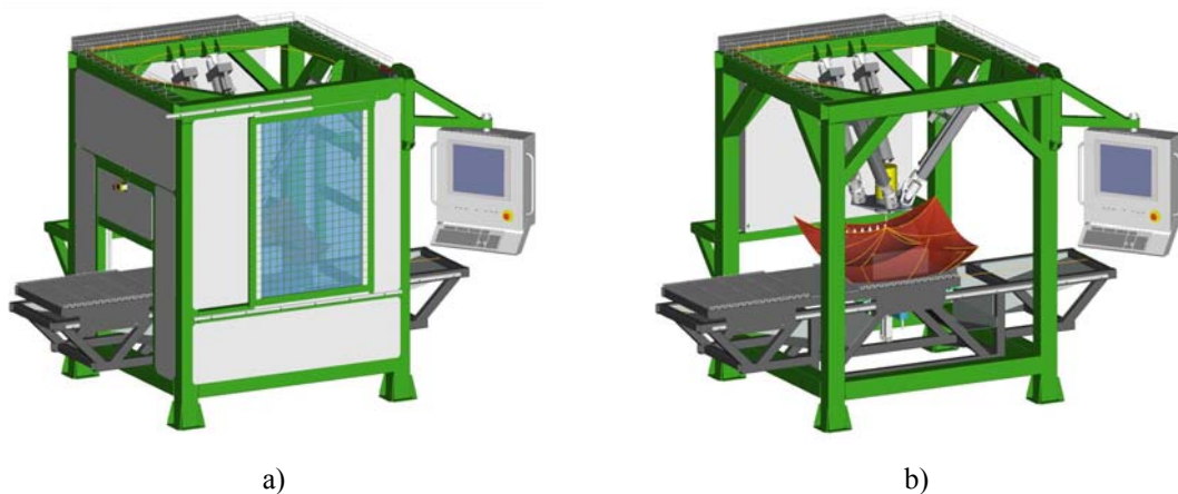
Figure 2. Design of a hexapod machine tool with (a) and without (b) cowling.
