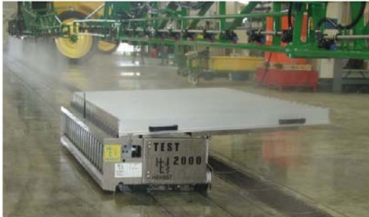
Figure 2. Mobile device for measuring the flow volume [4]
