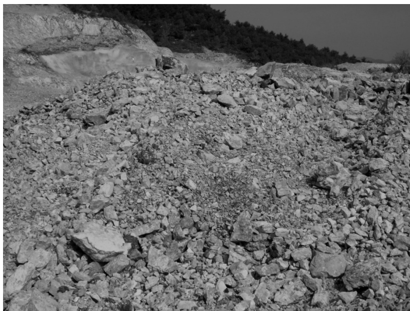
Figure 1. Fragmentation of the blasted material
