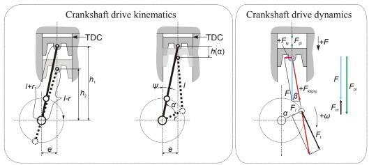
Figure 2. Kinematics and dynamics of the crankshaft drive
