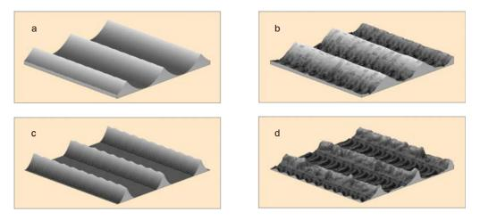
Figure 1. Surface topography for  $f=0.05 \text{ mm} \cdot tooth^{-1} \cdot revolution^{-1}$  and Rd=0.40 mm, for E=0.001: a) simulated, b) experimental, and for E=0.100 mm: c) simulated, d) experimental
