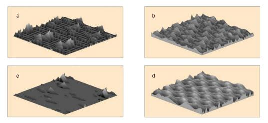
Figure 3. Surface topography for  $f=0.40 \text{ mm}\cdot\text{tooth}^{-1}\cdot\text{revolution}^{-1}$  and Rd=0.05 mm, for E=0.001: a) simulated, b) experimental, and for E=0.100 mm: c) simulated, d) experimental
