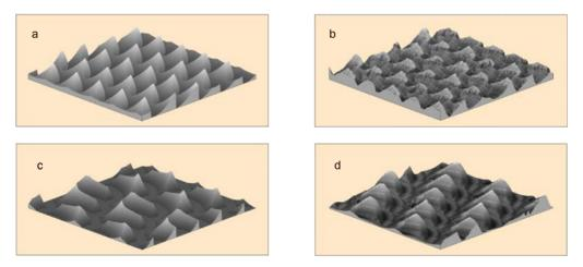
Figure 2. Surface topography for  $f=0.20 \text{ mm} \cdot \text{tot} \text{h}^{-1} \cdot \text{revolution}^{-1}$  and Rd=0.20 mm, for E=0.001: a) simulated, b) experimental, and for E=0.100 mm: c) simulated, d) experimental
